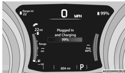
High Voltage Battery Display
